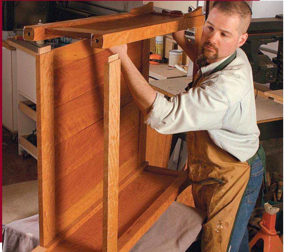
Top off the assembly with the final side. Use pine blocks on each side of the corbels to transfer clamping pressure to the posts.
